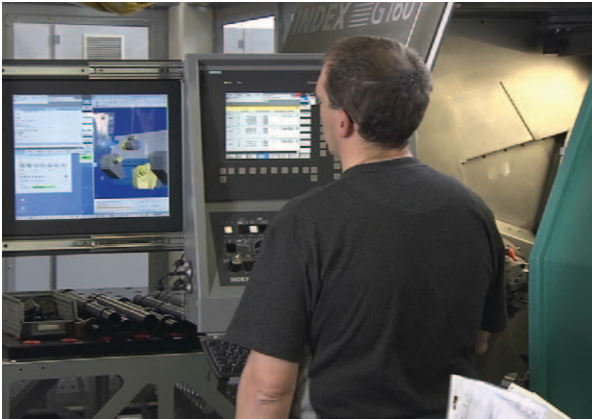
Figure 7: Machinists can verify NC programs and machine setup for the next job by using the virtual machine without tying up the physical machine tool.
