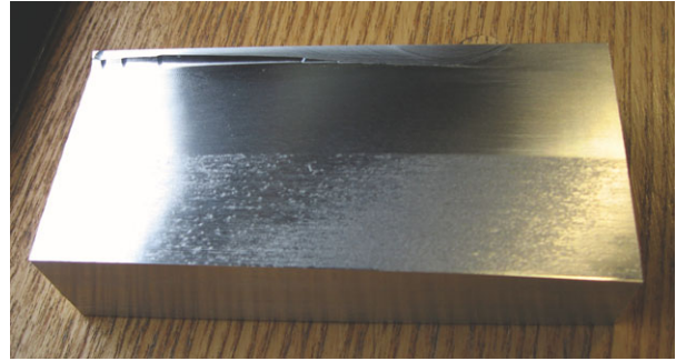
Figure 2: Uniform point distribution (top half of block) results in better surface finish compared to points distributed "out of step" on adjacent passes (bottom half of block).
